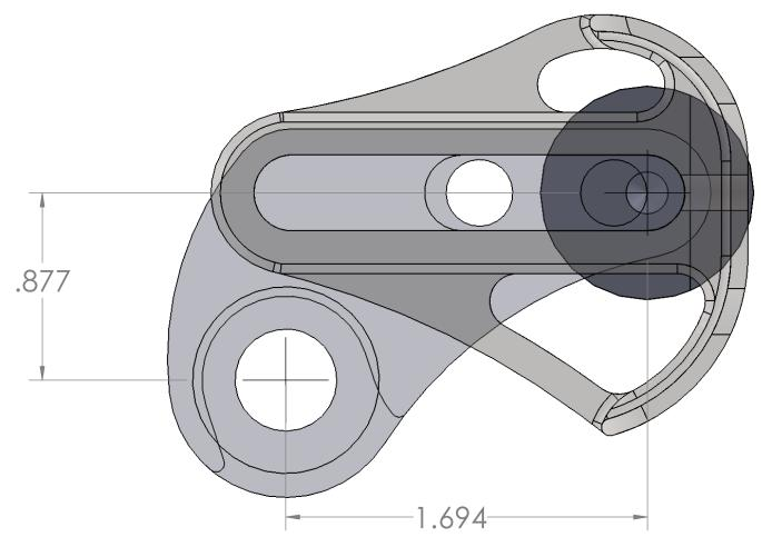
These dimensions are from dummy axle centerline to insert axle centerline all the way forward on frame piece
