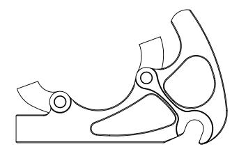
ADAPTER PROFILE MUST MATCH DROPOUT PROFILE, NO ENGRAVE VISIBLE FROM THIS VIEW
