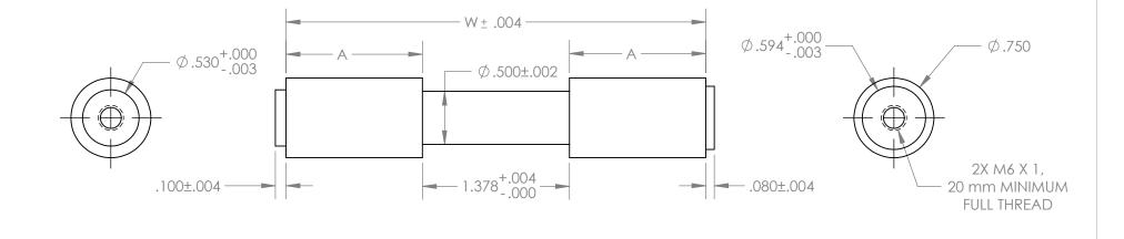
**PARAGON MACHINE WORKS** TITLE: NAME DATE 15 mm, FRONT, SPACER 4/20 CN DRAWN BY: 4/20 PROPRIETARY AND CHECKED BY: ΜN CONFIDENTIAL MATERIAL: GENERAL TOLERANCES: THE INFORMATION CONTAINED IN THIS DRAWING IS PROVIDED FOR FRAMEBUILDERS AND IS THE PROPERTY OF PARAGON MACHINE WORKS, ANY SIZE DWG. NO. REV X.X ± 0.020" 02 27 A Α X.XX ± 0.010" REPRODUCTION IN PART OR AS A WHOLE X.XXX ± 0.005" WITHOUT THE WRITTEN PERMISSION OF PARAGON MACHINE WORKS IS PROHIBITED. SCALE: 2:3 SHEET 1 OF 1
